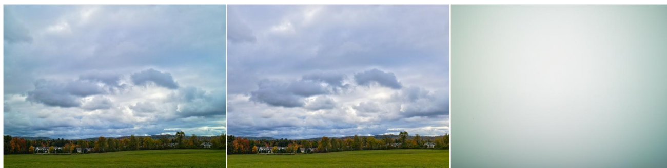
Example of the flat field correction. Image before, image after correction and the flat field file used. Notice the correction of both luminosity and color non-uniformities.
